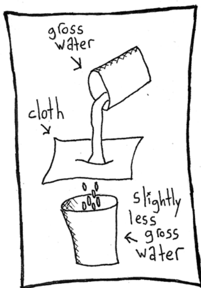
Figure 2-4: (bottom) a gravity-fed home-made water Filter. If the source of Water is above the Filter, then Water will flow.
